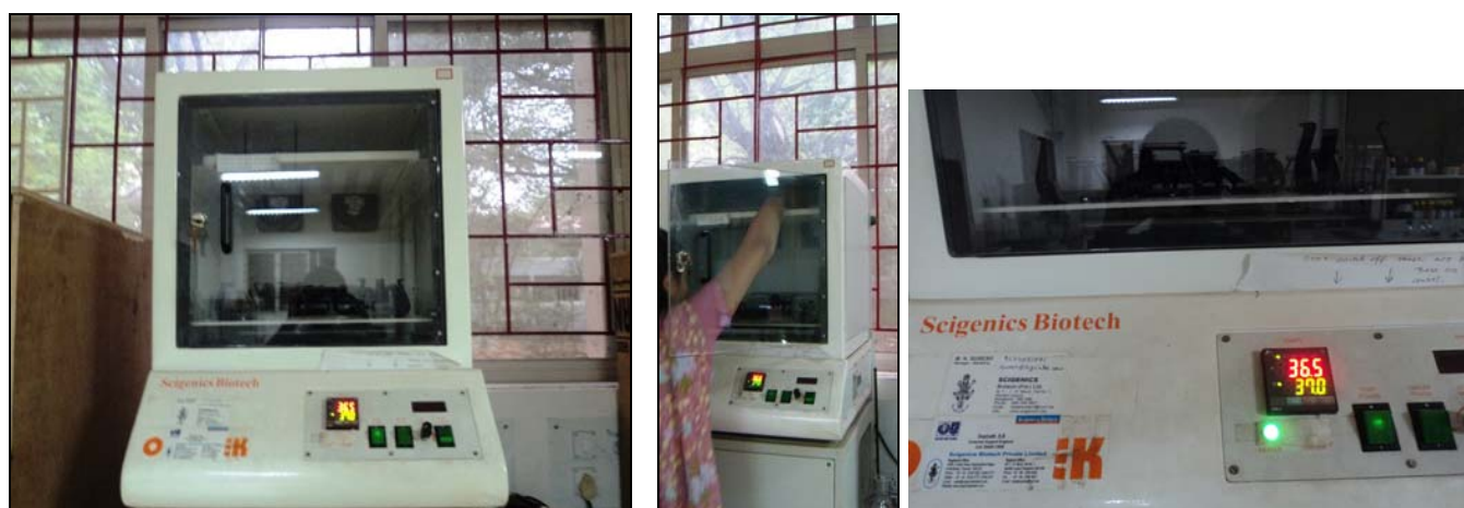
Figure 17: Inoculated samples are kept for incubation for 24 hours at 37°C
