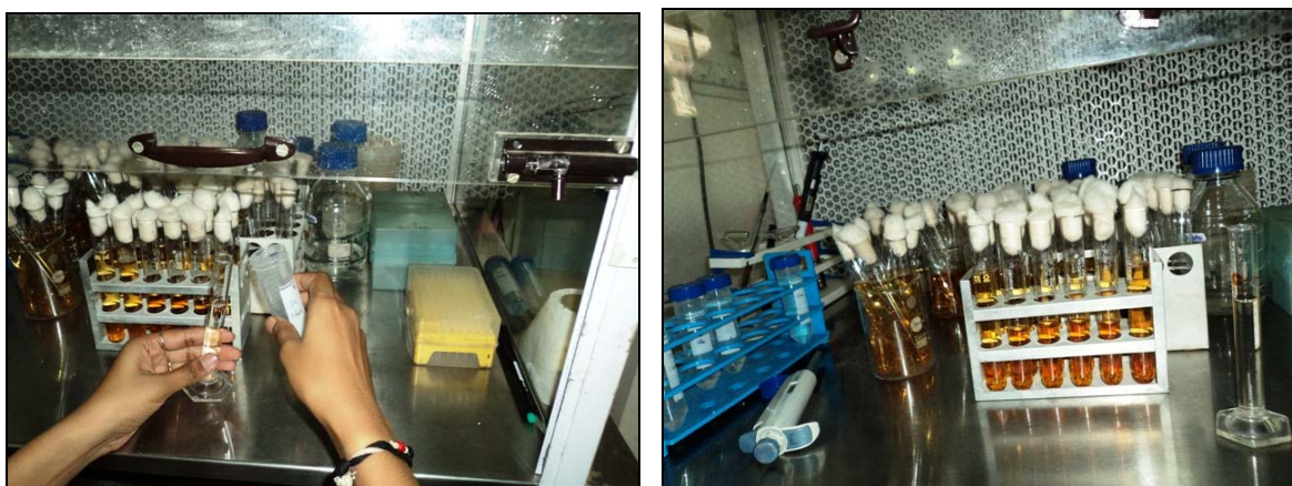
Figure 19: Known quantity of water sample inoculated in sterilized test tubes and kept aseptically inside the laminar air flow chamber
