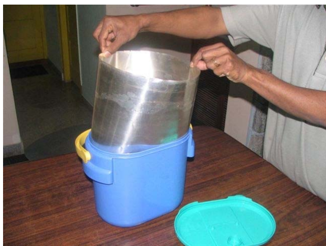
Figure 3: Container with silver sheet immersed inside the water sample
