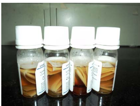
Figure 11: Change in color of H 2 S vials, color less vials indicate non-contaminant water black color indicate contaminated water
