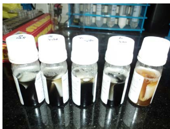
Figure 11: Change in color of H 2 S vials, color less vials indicate non-contaminant water black color indicate contaminated water
