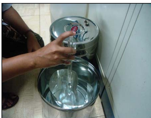
Figure 12: Sample kept in stain less steel container with silver sheet
