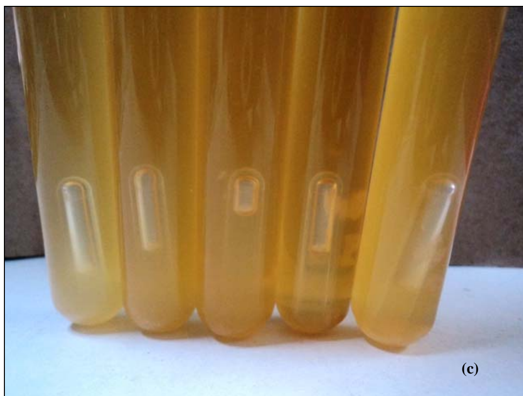
Figure 20: (a) Test tubes observed - all 5 positive tubes – raw water 10mL sample (b) Test tubes observed - 4 positive tubes – raw water 1mL sample (c) Test tubes observed - 4 positive tubes – raw water 0.1mL sample Positive 5 – 4 – 4 tubes indicate 350MPN/100mL
