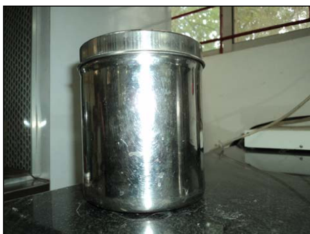
Figure 9: 1 litre capacity SS drum – 15.5cm(D) x 18cm(H)
