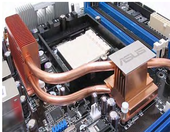
Figure 1.6 Heat Pipe Assembly Used in Mother Board
