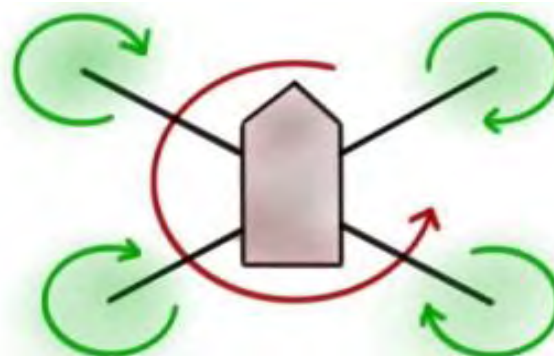
Fig 1.3.3: When the rotors spin clockwise, the multirotor would start spinning uncontrollably in a counterclockwise direction.
