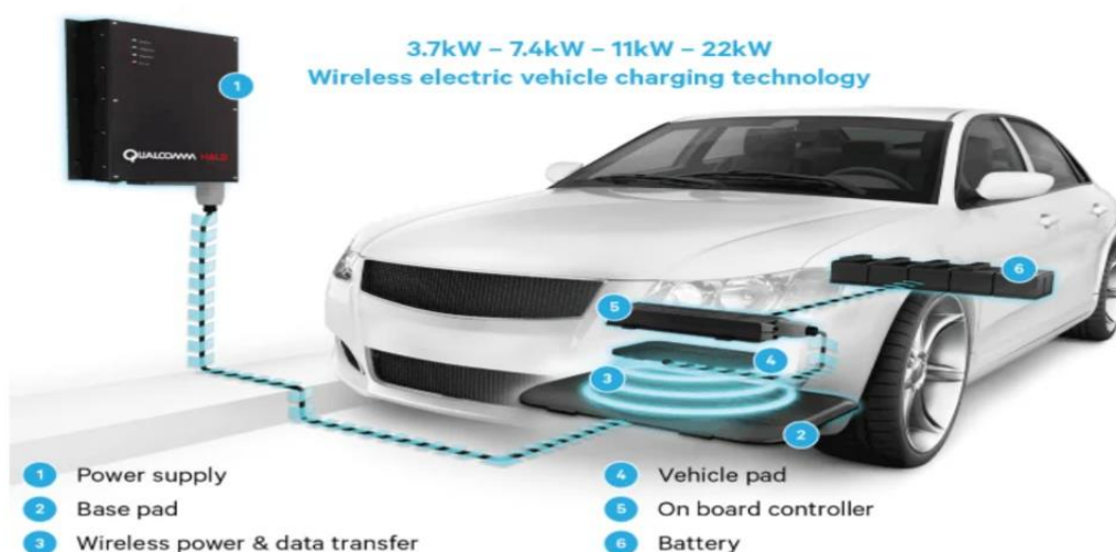
Figure 1: IoT- Enabled Static Wireless charging for Electric Vehicles
