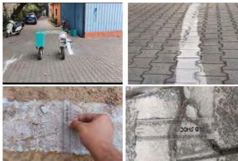
Figure 3: Painting Result (150 mm width)
