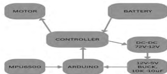
Figure 3: System Flow Block Diagram.
