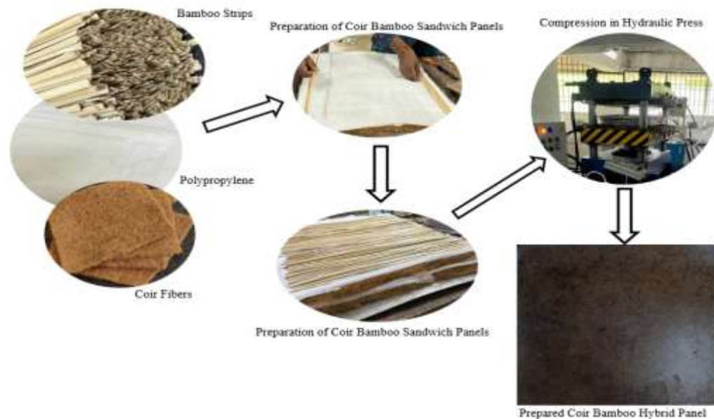
Figure 1: Fabrication Process of Hybrid Panels
