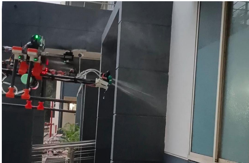
Figure 2: Drone Cleaning a Window
