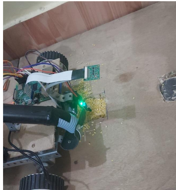
Fig.7 working model successfully detects the first 2cm pothole using sensors, initiating the filling process with high accuracy and efficiency.
