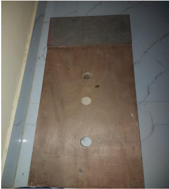
Fig.6 illustrates the road model features potholes of 2cm, 4cm, and >7cm depths to evaluate detection, filling, and system response.
