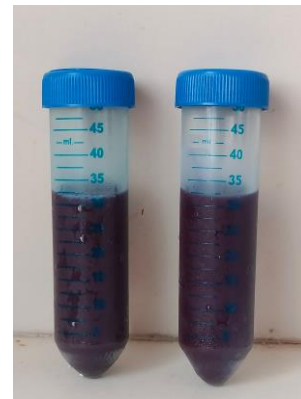
Figure 8: Supernatant obtained using 100mM phosphate buffer (pH 7)
