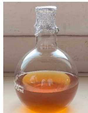
Figure 6: Oil-solvent mixture obtained after soxhlet extraction
