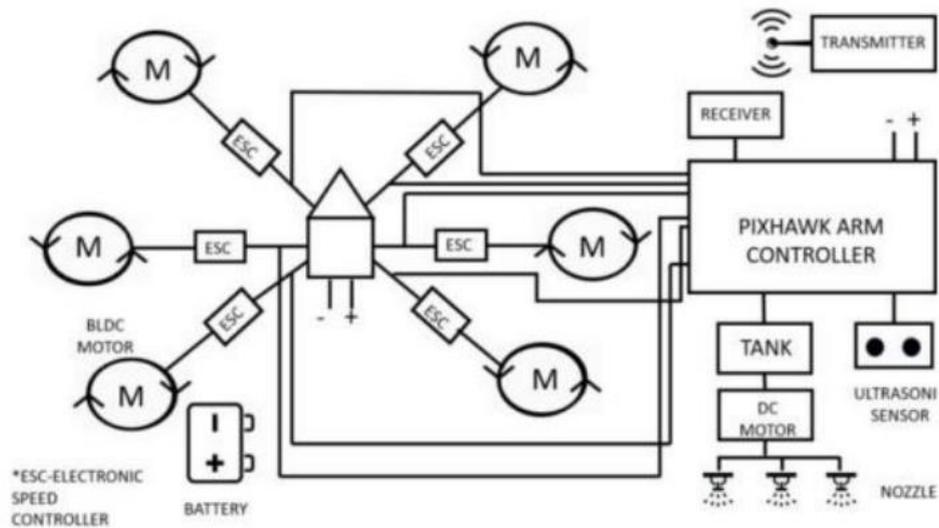
The main goal of this research is to create an effective hexacopter system with a built-in payload configuration. The remote control can be used to activate the spraying mechanism. Figure 1 shows the system's whole building block. To build the physical model of drone these were some of the steps which were followed, which are given below:
