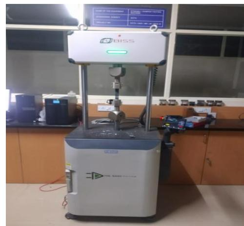
Figure 5 UTM used for tensile test
