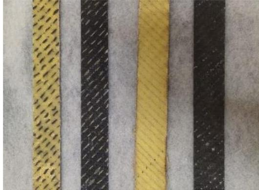
Figure 6 - Flexural Test Specimens
