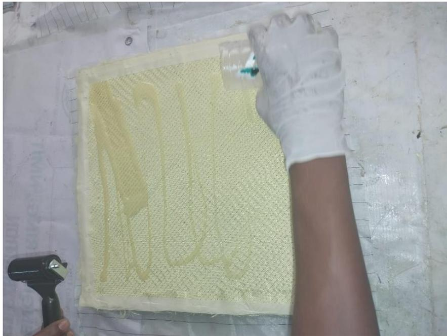
Figure 2 - Hand Lay Up Process.
