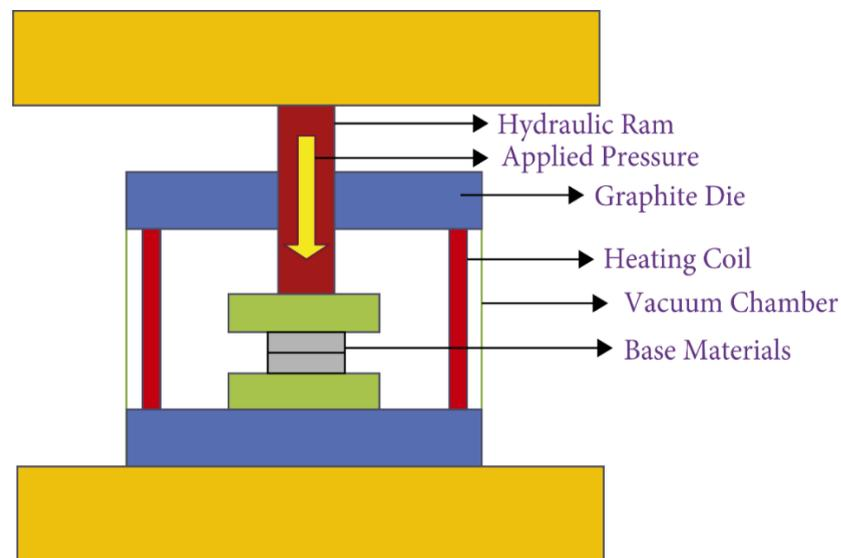
**Figure 3.1: Schematic representation of diffusion bonding process
