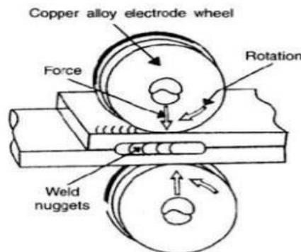
**Figure 1.5: Seam Welding**
