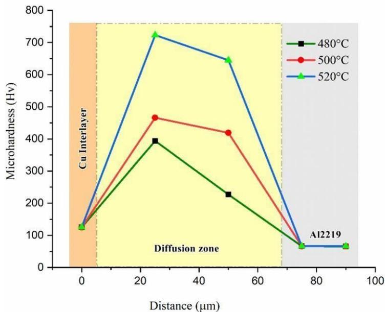
Fig.4.6 Micro hardness profile across the TLP bonded joints
