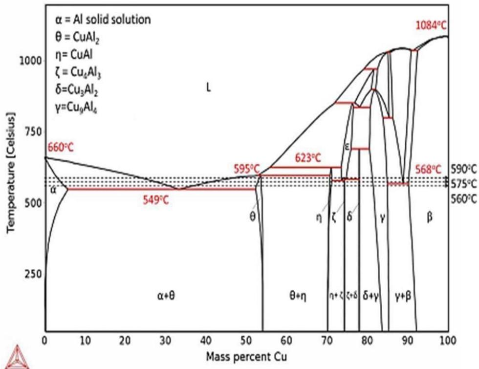
Fig. 4.2 Calculated Al-Cu binary phase diagram [27]
