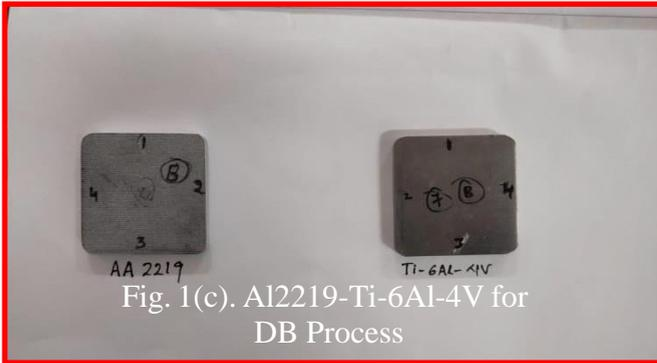
Fig. 1(c). Al2219-Ti-6Al-4V for DB Process
