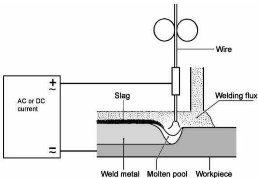
**Figure 1.2: Submerged Arc Welding**
