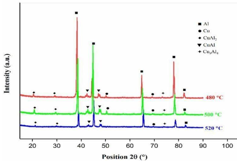
Fig.4.4 XRD pattern for the specimens bonded at 480, 500 and 520 °C
