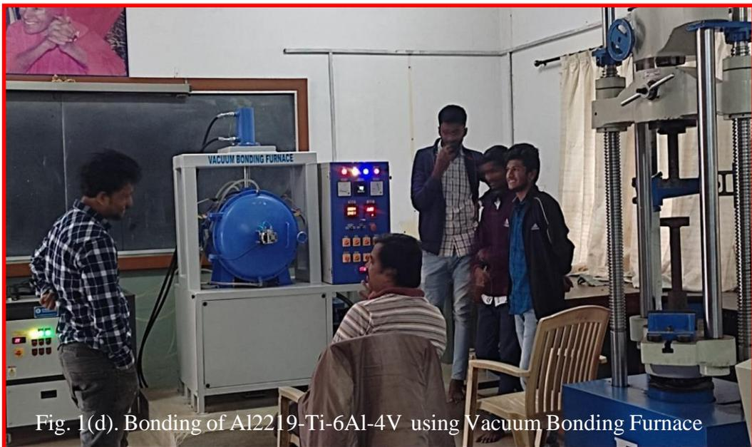
Fig. 1(d). Bonding of Al2219-Ti-6Al-4V using Vacuum Bonding Furnace
