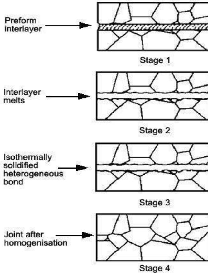
Figure 1.1.1: Transient liquid phase bonding
