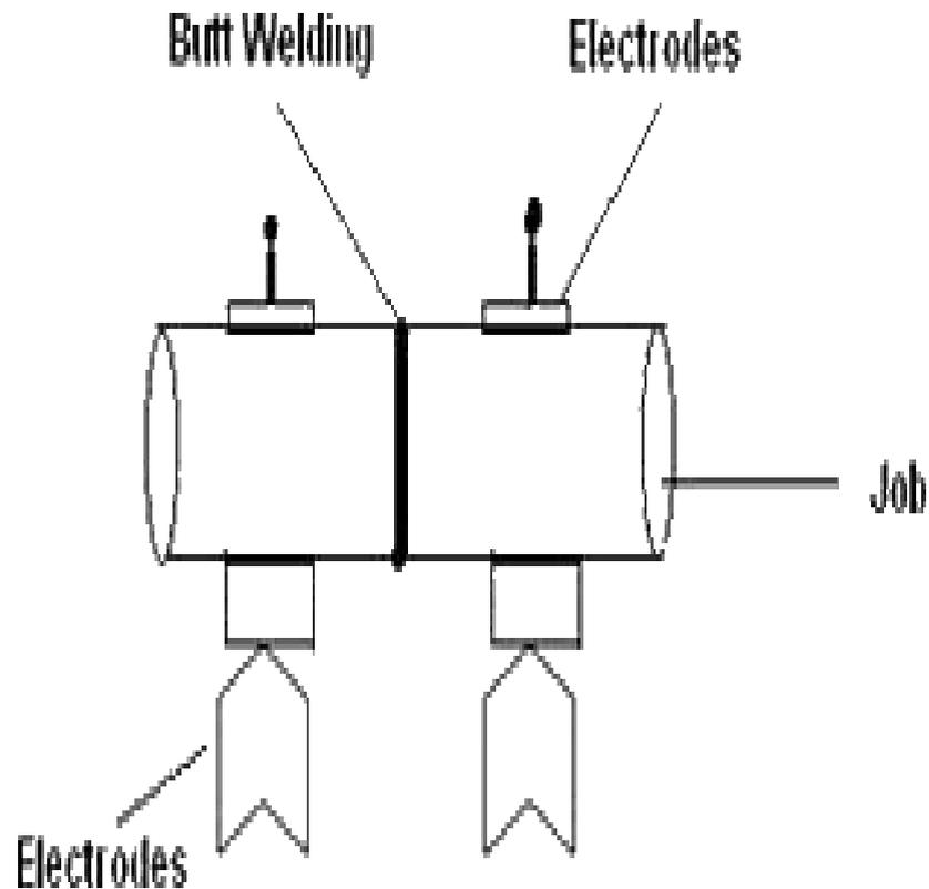
**Figure 1.6: Resistance Butt Welding**
