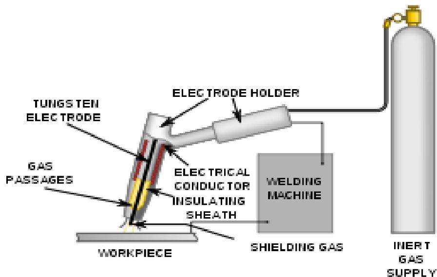
Figure 1.1: Gas Arc Welding
