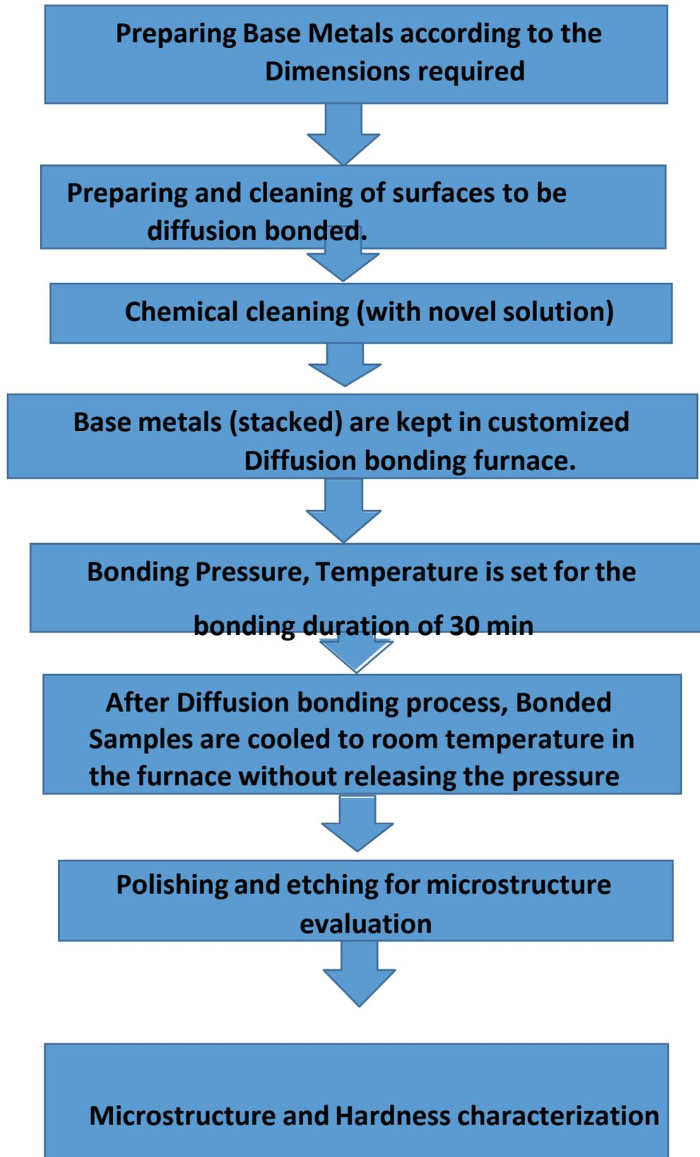
**Figure 3.2: Diffusion Bonding Methodology**
