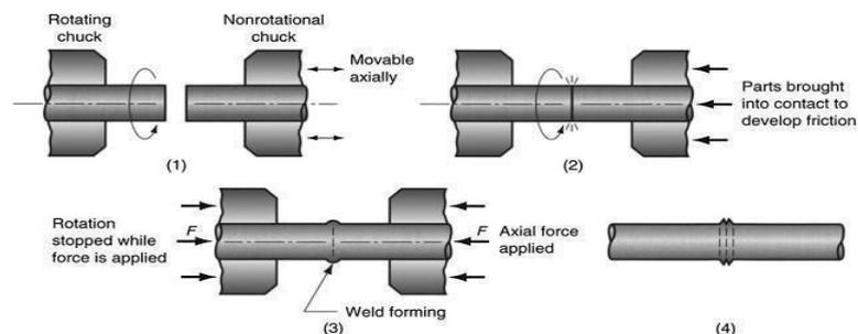
Figure 1.8: Friction Welding
