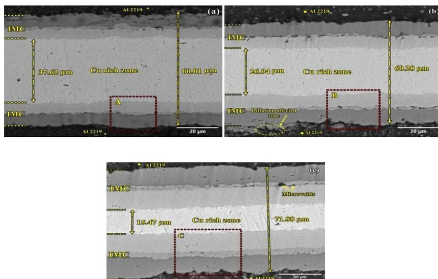
**Fig.4.1 BSE images of diffusion bonded specimens at (a) 480 °C (b) 500 °C (c) 520 °C**
