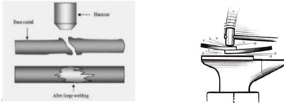
Figure 1.7: Forge Welding
