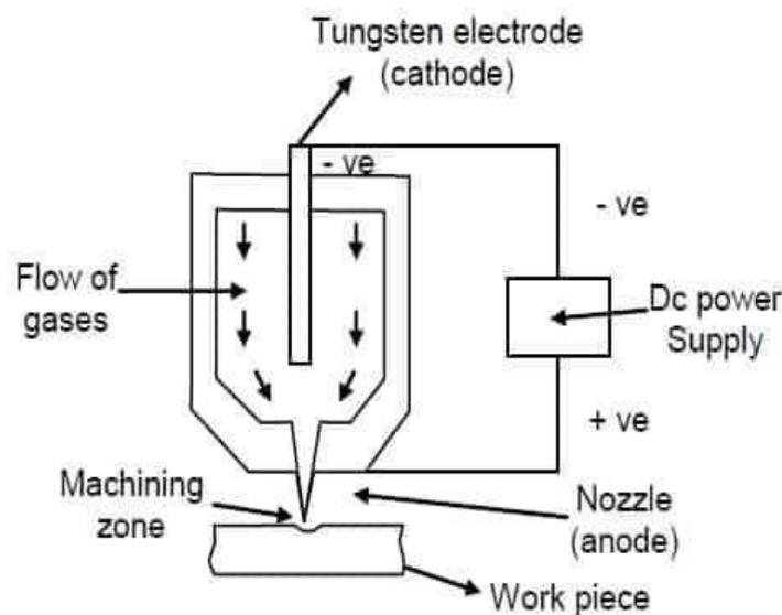
**Figure 1.3: Plasma Arc Welding**
