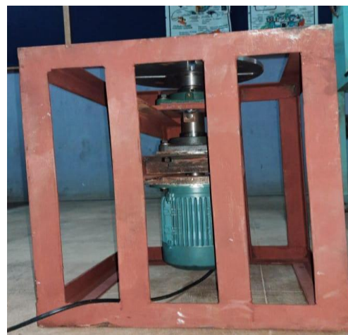
Figure 3 Side View of Centrifugal casting machine
