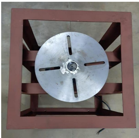
Figure 2. Top View of Centrifugal casting machine
