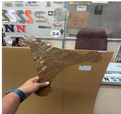
Figure 11: composite drone frame
