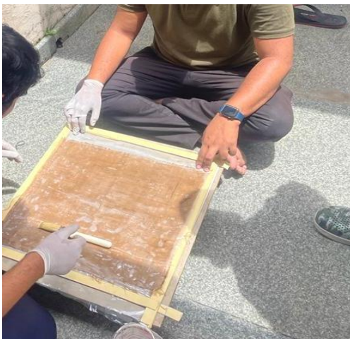
Figure 10: hand-layup process fabrication
