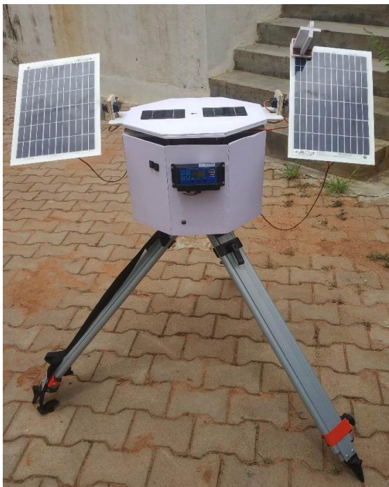
Fig: Setup of Portable Automatic Dual Axis Solar Tracker
