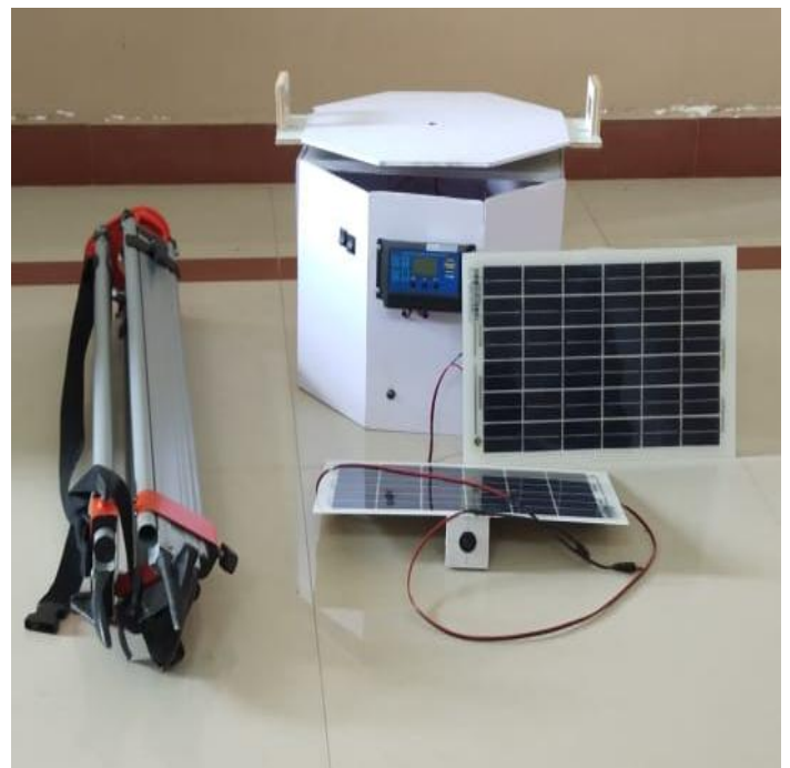
Fig: Setup of Portable Automatic Dual Axis Solar Tracker
