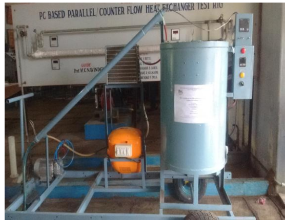
Fig 4: Fabricated Pyrolysis Unit
