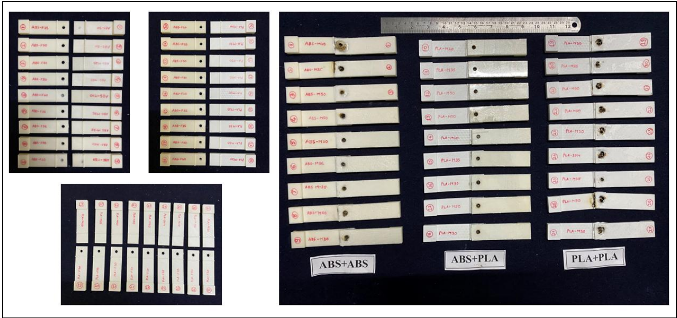
Figure 3: Microwave welded specimens of different material combinations
