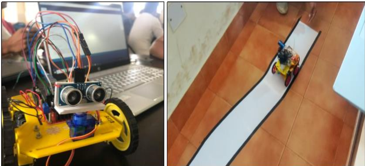
Fig 6 and 7: Collision avoidance system using ultrasonic sensor Car prototype demonstrating lane assist technology
