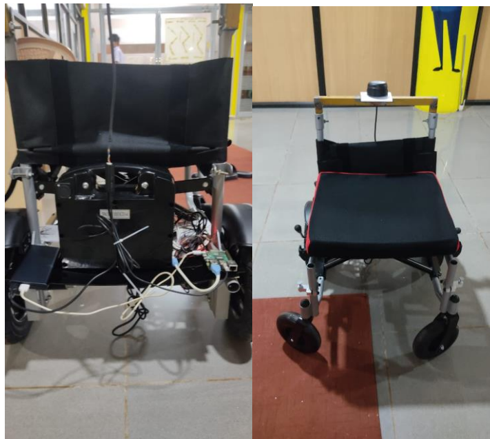
Fig. 8 Back and Front view of the autonomous carrier robot
