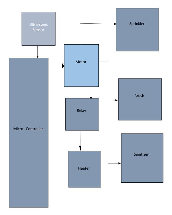
Fig 1.1 Block Diagram of Automatic commode seat
