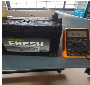
Fig: Output voltage test of battery
