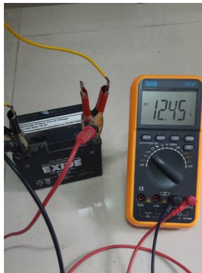
Fig: Bicycle battery voltage when Charging
