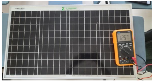
Fig: Open circuit voltage test of solar panel with multimeter when sun radiation is low
