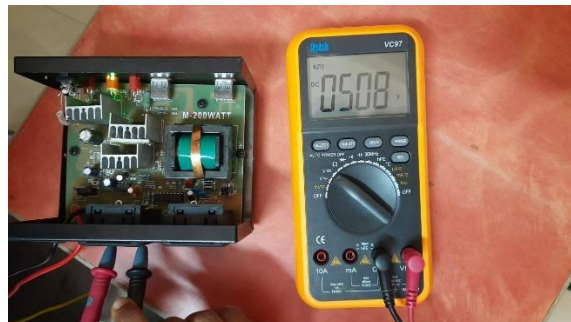
Fig: output voltage test of dc-dc boost converter with multimeter
