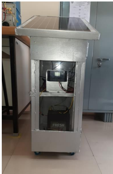
Fig: Solar based charging station
