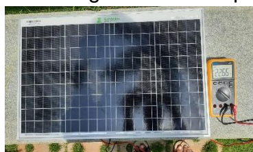
Fig: Open circuit voltage test of solar panel with multimeter when sun radiation is high
