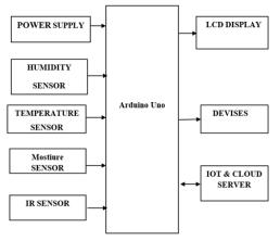
IOT and Arduino Based Industrial fault detection system sends the signal from different sensors, i.e. Humidity, Air Pressure, Temperature and LPG gas sensor to the micro-controller – Arduino. The micro-controller then sends this data to the IOT module (ESP8266). ESP8266 is a chip used for connecting micro-controllers to Wi-Fi network and make TCP/IP connections and send data.
