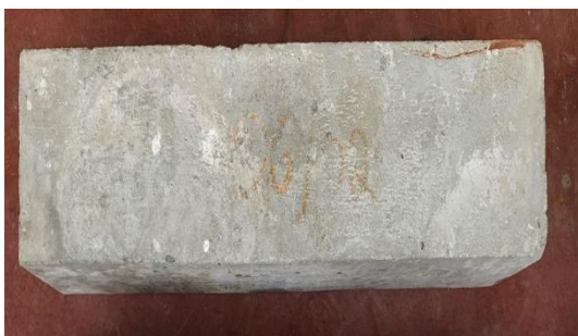
Fig. 2: Control beam (unstrengthened beam)
