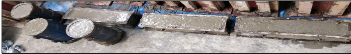
Fig 8. Casting cylinders and prisms
