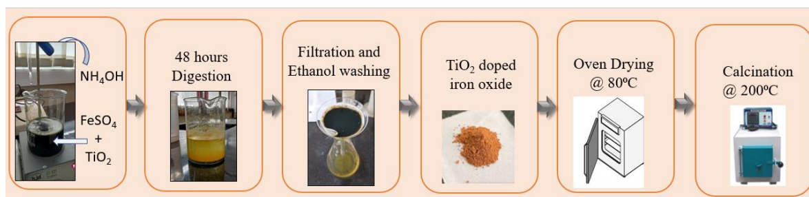
Fig: 2 Graphical abstract of synthesis of Fe-Ti bimetal oxide nanoparticle
