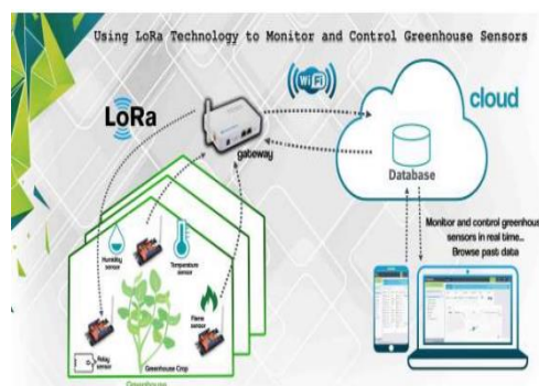
Fig.1. Smart Monitor and Control for Greenhouse Sensors System
