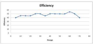
The efficiency of the coagulant in removing the turbidity of the sample is highest whenthe dosage is equal to 60ml which is the optimum dosage.
