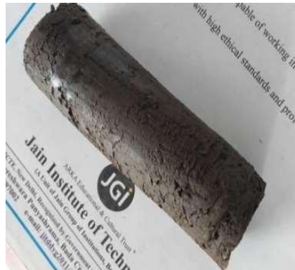
Figure 1: Unconfined compressive strength test specimen
