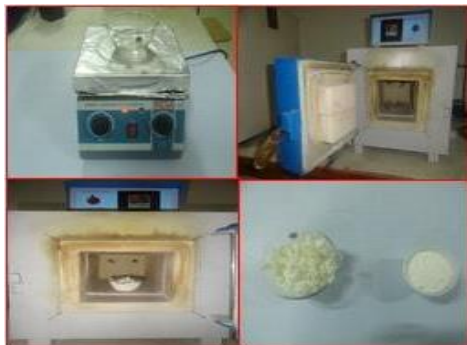
Figure 1: Synthesis of nanoparticles by solution combustion method
