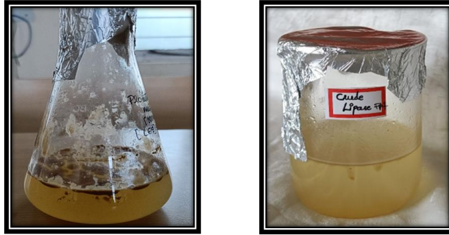
Figure: 2) submerged Fermented production media consists of bacteria ( Lysinibacillus macroides FS) producing lipase. 3) crude lipase obtained after centrifugation
