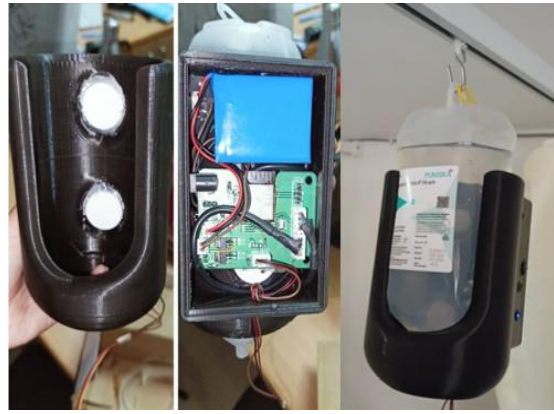
IoT Based Smart System for Monitoring and Control of IV (INRAVENOUS) Fluids for Patients
